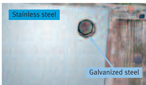
Figure 10a, 10b: Practical examples of the principle shown in Figure 9 (galvanized carbon steel in contact with stainless steel, in a marine atmosphere)
