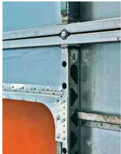
Figure 24: In this side wall of a commuter train, the structure and outer panels are in different grades of stainless steel. As these have identical potentials, no galvanic corrosion can occur.
