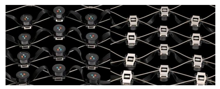
Single LED-LINES (max. 56 single LED-DOTS on ribbon cable) are fixed with stainless steel clamps on a stainless steel mesh with rope-Ø 2,0mm. The mesh width can vary between 60 and 300mm. The size of the X-LED MESH is not limited, because several mesh parts can be connected smoothly together.
